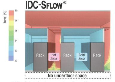
■ Rack intake temperature is uniform, and closer to supplied-air temperature.
