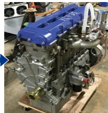
Built-in engine (3,500cc (four cylinders))
